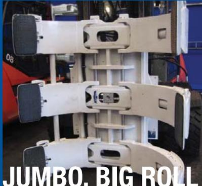
High-production roll clamp for wide printing paper handling of kraft, linerboard and coated stock.
