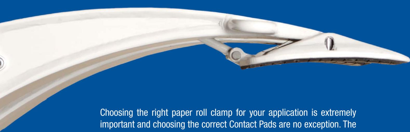
Choosing the right paper roll clamp for your application is extremely important and choosing the correct Contact Pads are no exception. The correct contact pads will optimize clamp force which ultimately results in reduced damage. Cascade is dedicated to making sure that your paper roll clamp comes optimized with the design features and accessories you need for your application.
