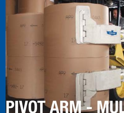
Designed for mills and stevedores where multiple roll handling improves productivity. For handling newsprint, coated stock, kraft and linerboard.
