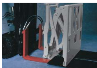
1. Position forks under platens.
