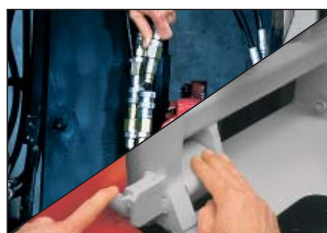
2. Connect quick change hydraulic couplers. 3. Engage lower hooks.
