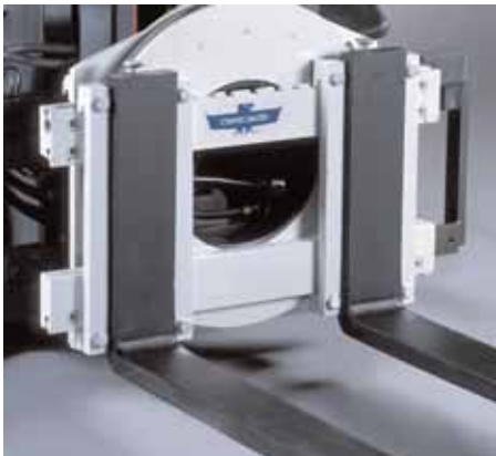
Fork Restraints to limit fork movement.
